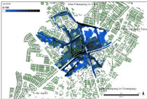
Figure 6 Local inundation of urban area due to combined influences of local rainfall and backwater effects from river flooding and/or storm surge and tide.
